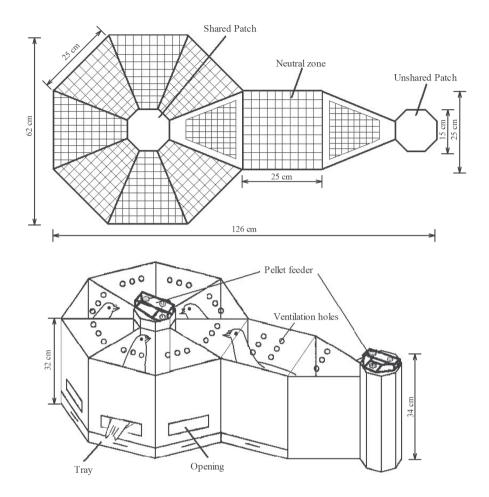
*Figure 1.* The operant chamber comprised three parts: a shared patch (left side), an unshared patch (right side), and a neutral zone. Microswitches were placed under the trapezoidal floor of each of the patches to detect the responses made by the pigeons.
