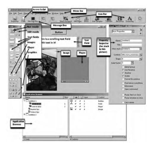
*Figure 2*. The LiveCode Environment showing the Tools Palette, the Application Browser, the Mainstack and the Property Inspector.
