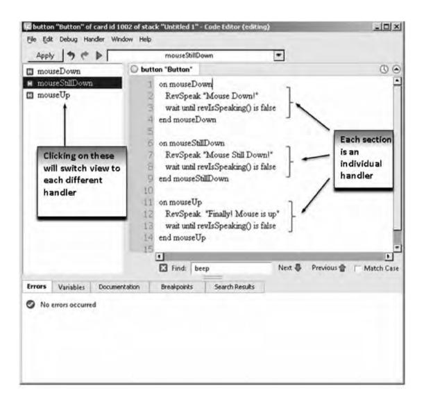
Figure 4. An example of three handlers in the script of a button.
